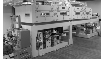
Fig. 5. R2R printing systems. (a)unwinding, (b)lateral controller, (c)infeeding, (d)preheating, (e)gravure printing, (f)drying unit, (g)cooling, (h)outfeeding, (i)rewinding
